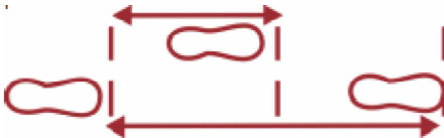
Figure 3. Illustration of a step and a pace. The longer is a pace (two steps).
